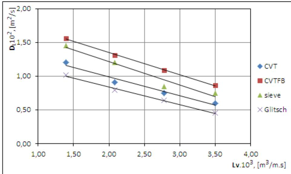
**Fig.2. Back-mixing coefficient in the liquid phase as a function of liquid flow rate per unit of bubbling area for the four different types of trays at vapour phase velocity 1.5 m/s**
