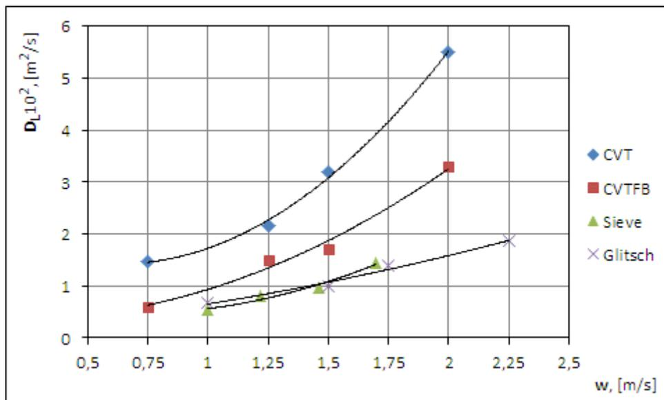
**Fig.1. Back-mixing coefficient in the liquid phase as a function of the gas velocity for the four different types of trays at liquid flow rate per unit of bubbling area  $2.08 \text{ m}^3/\text{m.s}$**
