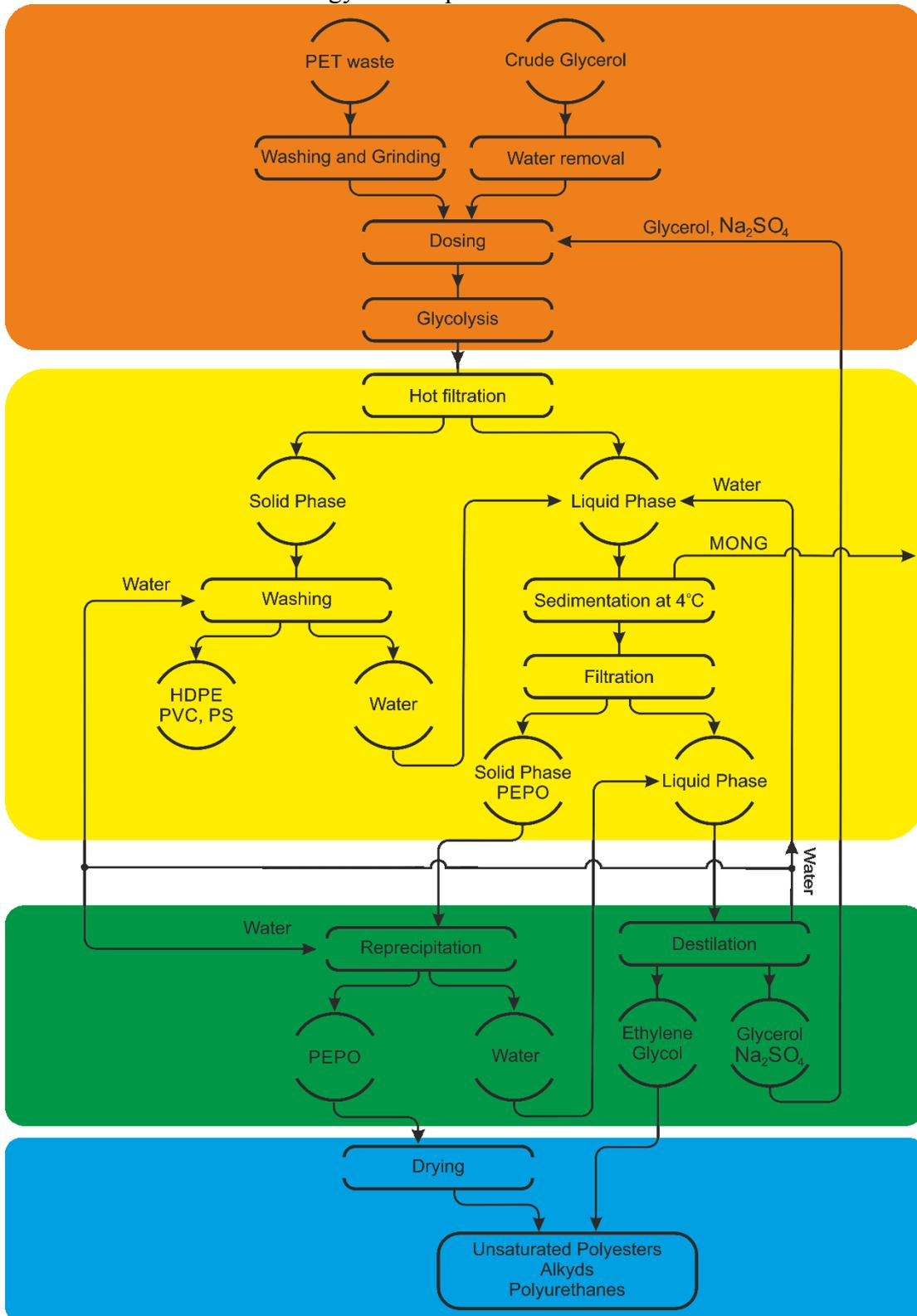
Scheme 2. Block diagram of the technology for utilization of waste PET by glycolysis with crude glycerol.
