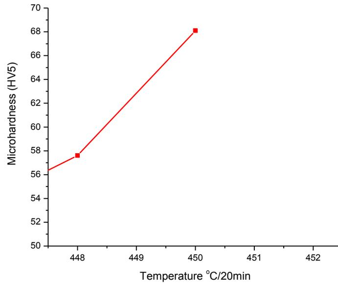
**Fig. 2.** Microhardness in function of temperature for equal treatment time
