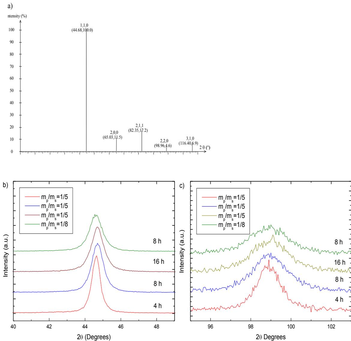
**Figure 1:** XRD a) peaks of un-milled Fe powders, b) (110) peaks of as-milled Fe powders, c) (220) peaks of as-milled Fe powders.
