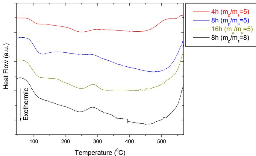
**Figure 3:** DSC trace of the as-milled Fe powders at a heating rate 10 K/min
