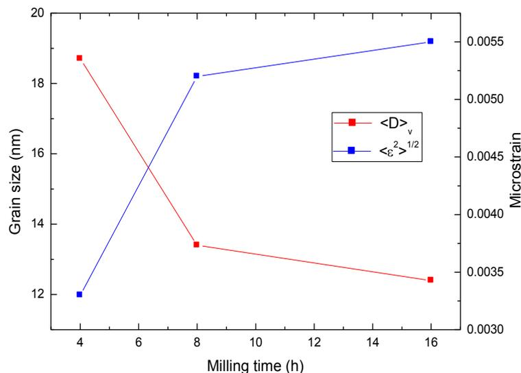
**Figure 2:** Evolution of the Grain size and microstrain in function of milling time (powder/sphere mass ratio 1/5).
