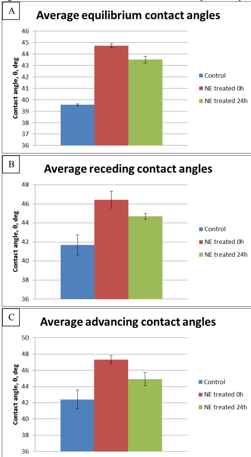
**Fig. 3** Contact angle measurements of the static (panel A), receding (panel B) and advancing (panel C) angles.
