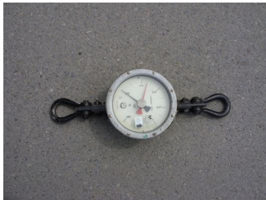
**Fig 4.** Dynamometer for determination of applied force
