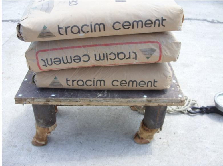
**Fig 3.** Tribometer for determination of coefficients of friction between hooves and floor (Phillips and Morris, 2000)
