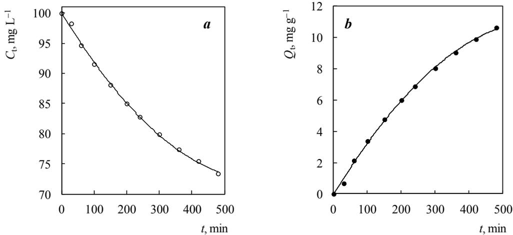
**Fig. 2.** Dependence of the concentration of Mn(II) ions in the solution (a) and the quantity of adsorbed Mn(II) ions (b) onto WRHA in relation to time.
