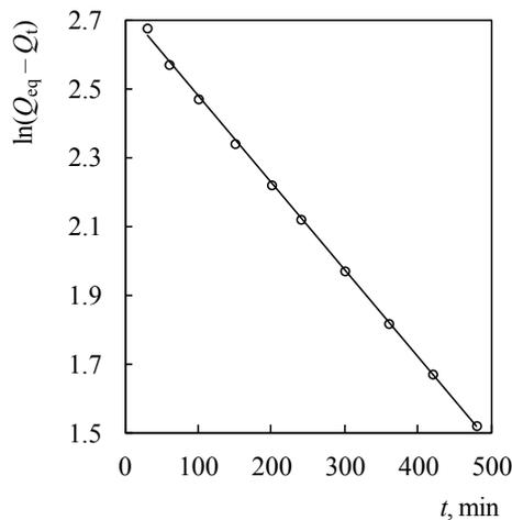
**Fig. 3.** Dependence of  $\ln(Q_{eq}-Q_t)$  versus  $t$  for adsorption of Mn(II) ions on WRHA.
