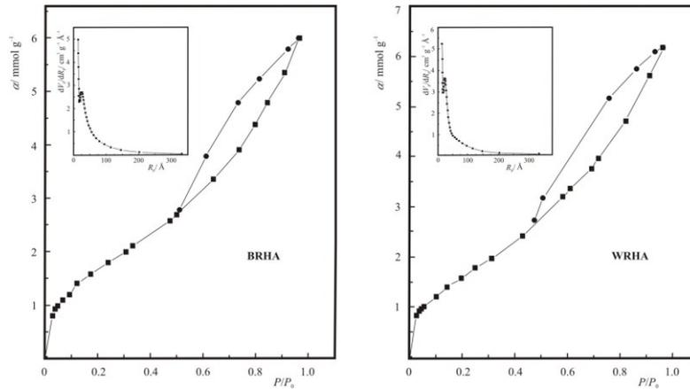
**Fig. 1.** Nitrogen adsorption isotherms of BRHA and WRHA and pore size distribution curves.
