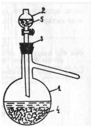
Fig.1. Hydrogen sulfide (carbon dioxide) obtaining installation:
