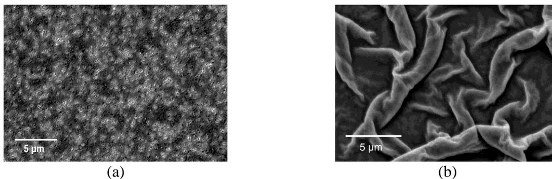
Fig. 1. SEM images of ZnO thin films annealed at 100°C (a) and 500°C (b).
