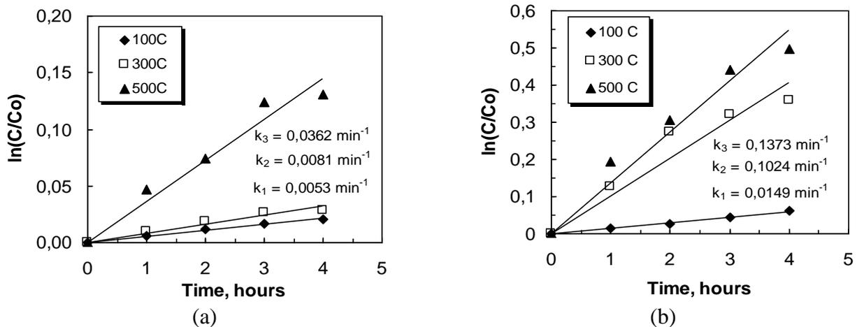
Fig. 3. Photodegradation curves of *Paracetamol* (a) and *Chloramphenicol* (b) using ZnO thin films as photocatalysts.
