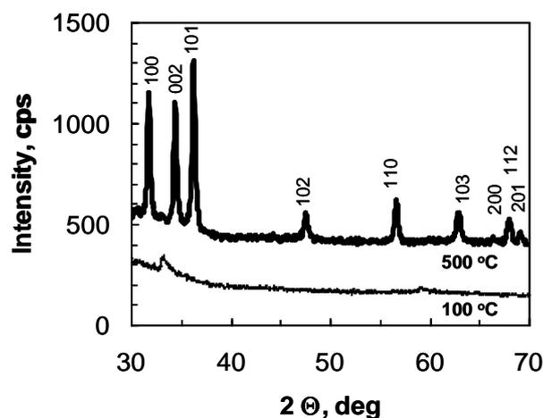
Fig. 2. XRD spectra of ZnO sol-gel films annealed at 100 and 500°C.
