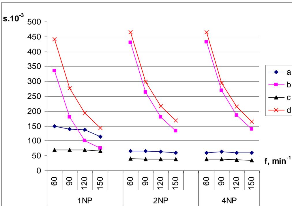
Fig. 2. Absolute values of the phases **a**, **b**, **c** and **d** of the pulsation system depending on frequency.
