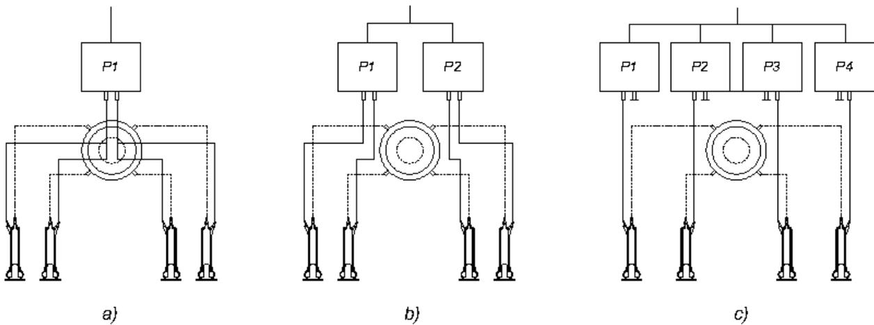
Fig. 1. Experimental set-up: a) experimental set-up of conventional pulsation system milking cluster (1NP); b) experimental set-up of milking cluster with 2 number of pulsators (2NP); c) experimental set-up of milking cluster with 4 number of pulsators (4NP).
