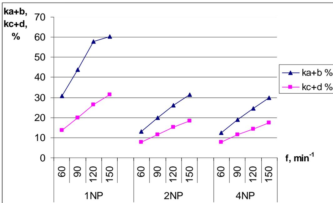
Fig. 3. Relative values of the phases **a**, **b**, **c** and **d** of the pulsation system depending on frequency.
