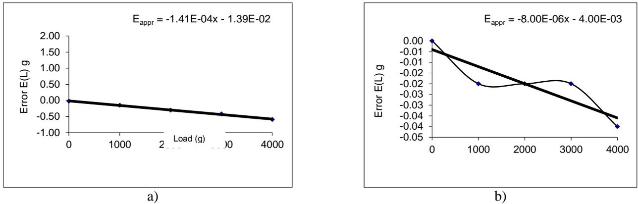
Figure 2. graphs of the indication errors of the weighing instrument before and after adjustment
