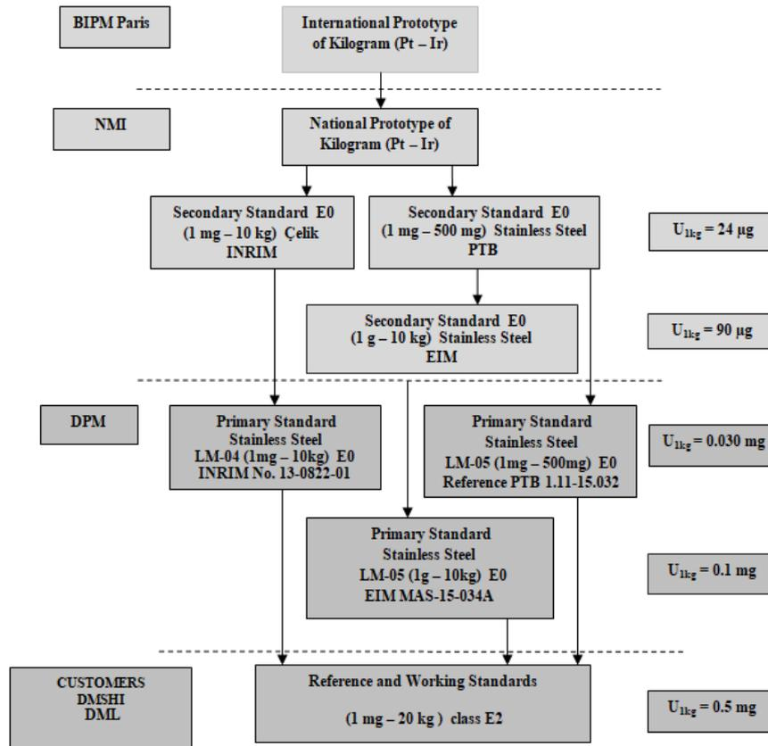
Figure 1. Traceability scheme for the mass unit in Albania 2016
