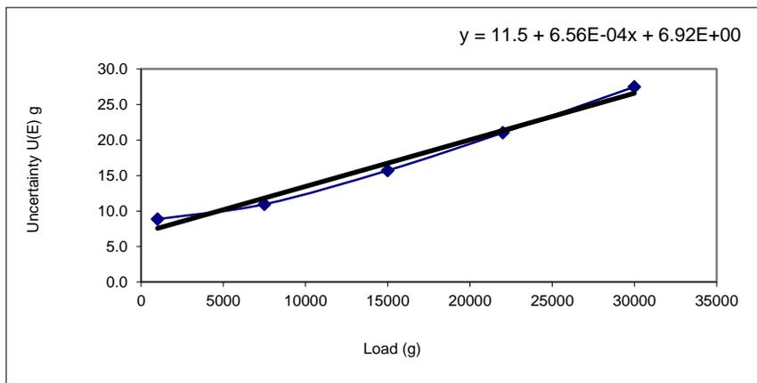
Figure 5. graph of the uncertainty of measurements after external adjustment
