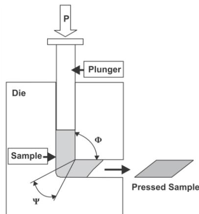
Fig. 3: Schematic view of an ECAP die
