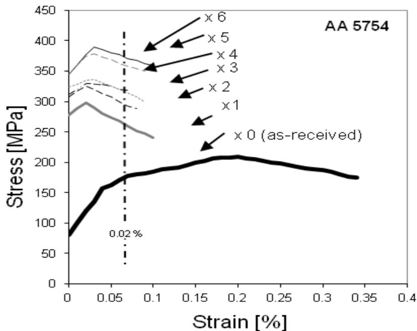
Fig. 7 Tensile test: stress versus strain of the AA 5754 at room temperature.
