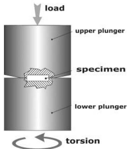
Fig. 1: Schematic, HPT set-up
