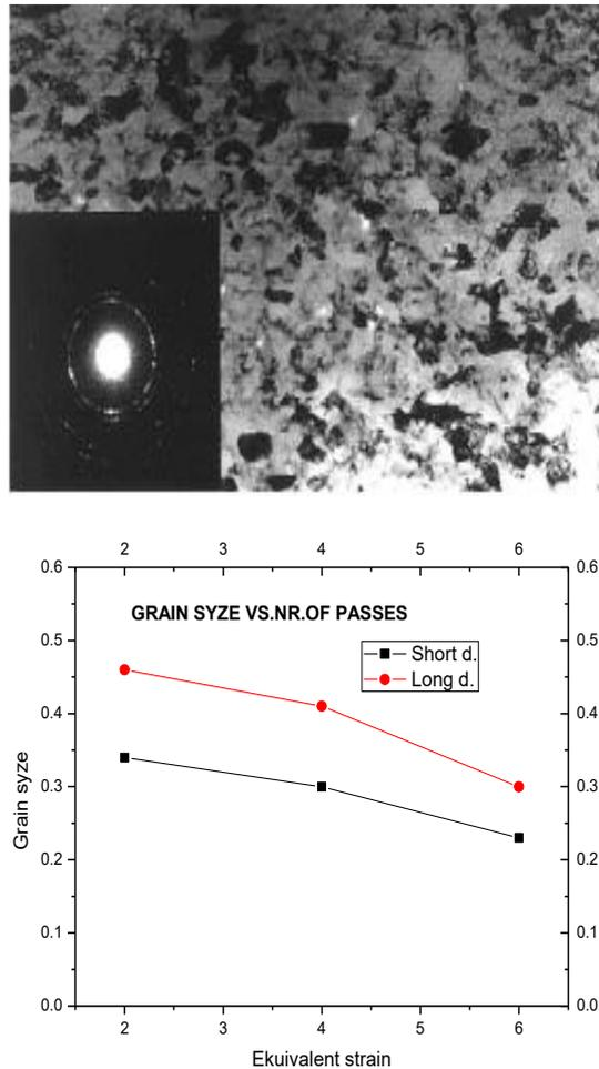
Fig.4. Microstructure observed TEM after ECAP through 4 passes. Grain size vs nr. of passes
