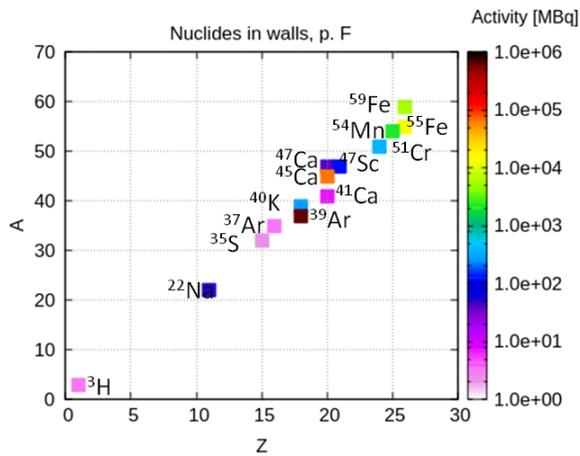
Figure 4a. Radionuclides for the target at position F.
