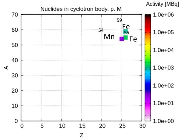
Figure 3b. Radionuclides in the cyclotron body for the target at position M.
