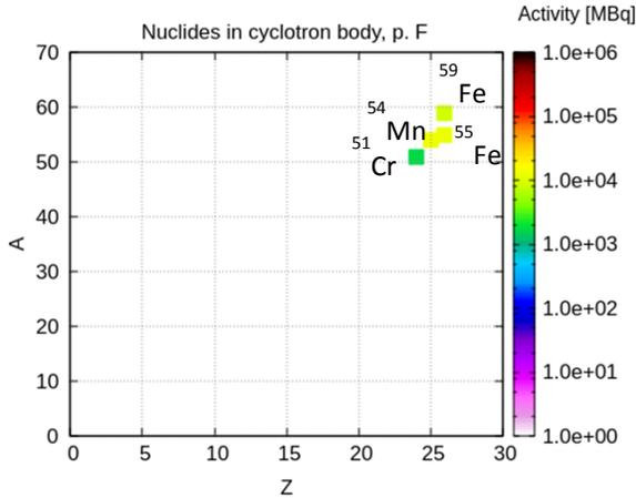
Figure 3a. Radionuclides in the cyclotron body for the target at position F.
