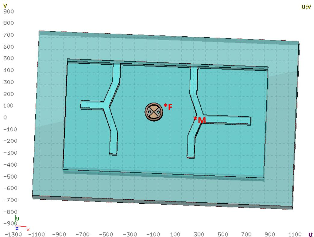
Figure 2. Top view of the vault with the cyclotron in the central part. The target for production of  $^{18}\text{F}$  is located at positions F or M. The axes dimensions are in centimeters.
