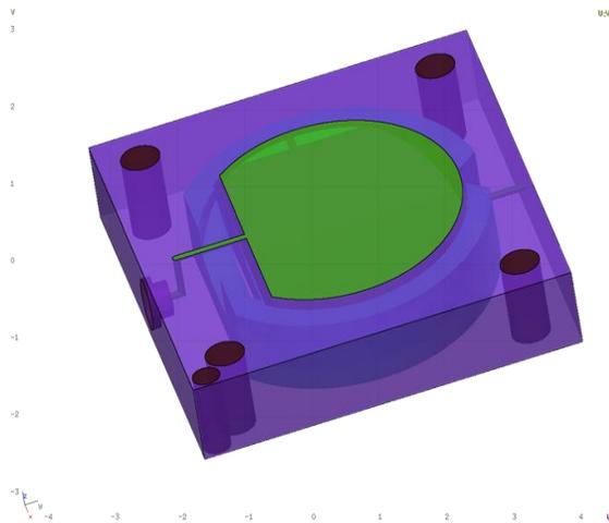
Figure 1a. Model of a high-current liquid target for  $^{18}\text{F}$  production. In green is the liquid volume. The proton beam impinges orthogonally to the target front surface.
