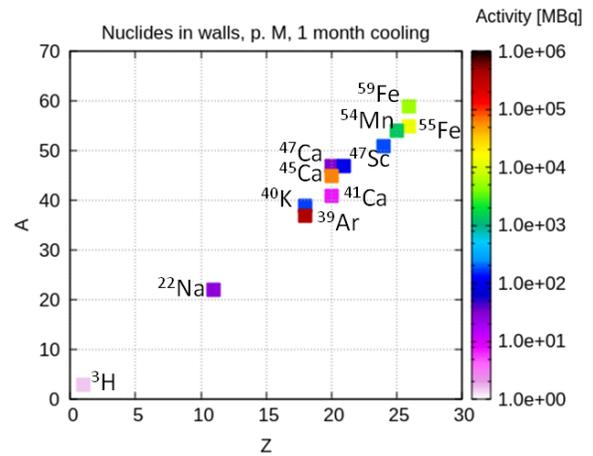
Figure 4b. Radionuclides for the target at position M.
