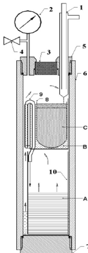
Figure 1: High pressure apparatus for Soxhlet extraction by liquid CO<sub>2</sub>: 1. Cooling finger, 2. Pressure gauge, 3. Window, 4. Valve, 5. Upper cover, 6. Steel cylinder, 7. Lower cover, 8. Extraction thimble, 9. Siphon, 10. Collection beaker, A. Product, B. Extract solution, C. Extraction material
