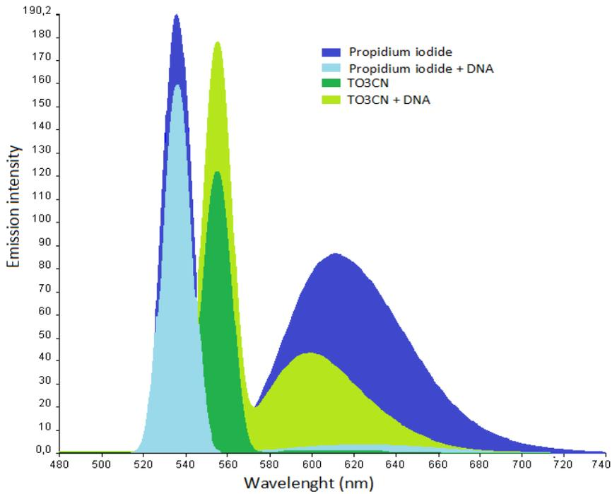
**Figure 2. Fluorescence spectra of PI and TO3CN before and after binding to DNA**
