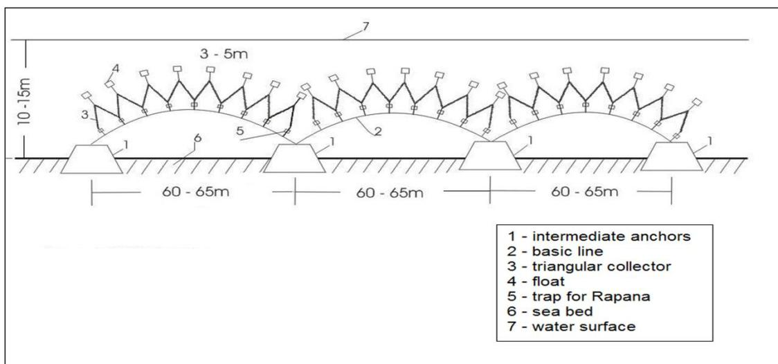
**Fig. 1.** Schematic diagram of one segment from the main line of the artificial habitat
