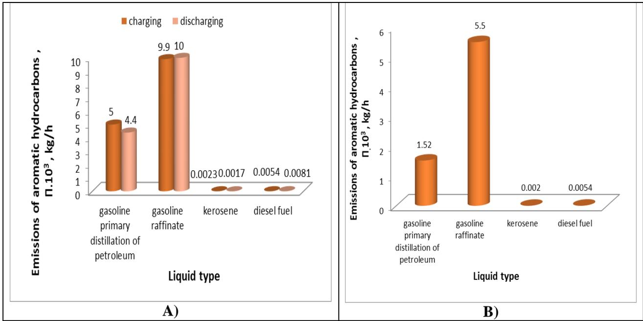
**Fig.2. Emissions of aromatic hydrocarbons (kg/h) from railway tank A)/storage tank B) charged with multicomponent liquids (petroleum products)**
