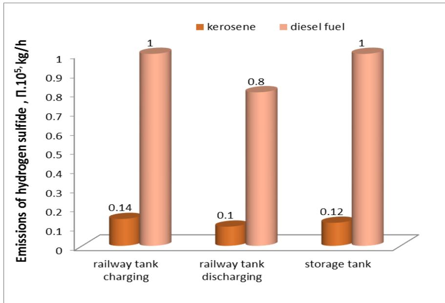
**Fig.3. Emissions of hydrogen sulfide (kg/h) released in the atmosphere from railway tank /storage tank charged with multicomponent liquids (petroleum products)**
