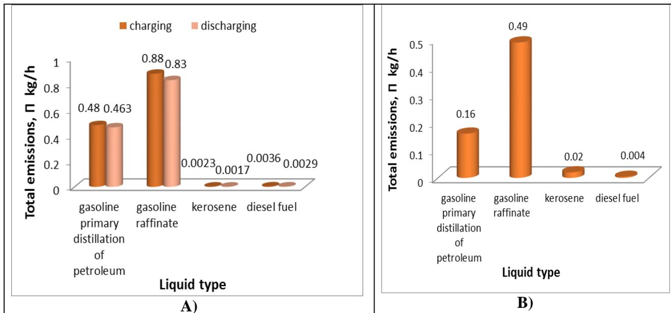
**Fig.1. Total emissions (kg/h) from a railway tank A)/storage tank B) charged with multicomponent liquids (petroleum products)**
